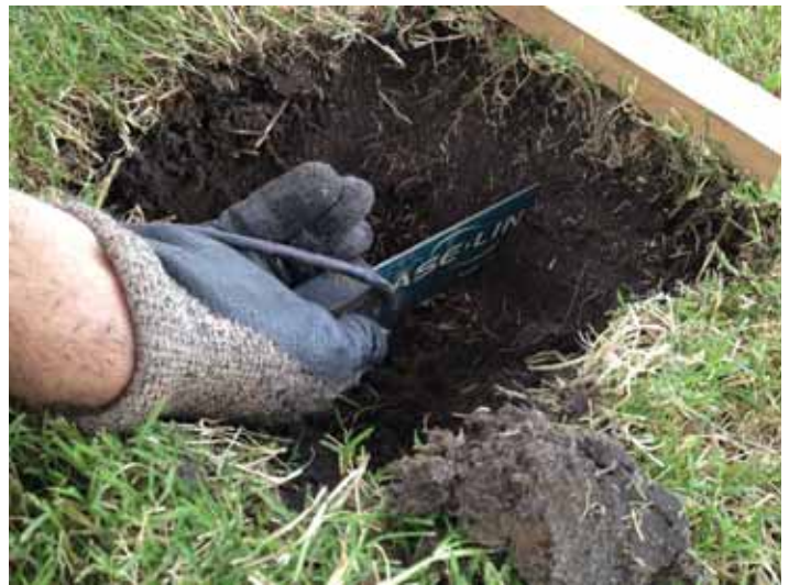
Figure 1. An example of a soil moisture sensor being installed in the soil.
